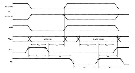
Figure 12. 8155/8156 Read/Write Timing Diagrams
